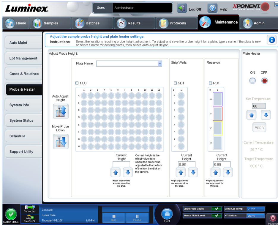
FIGURE 33. Sample Probe Height Adjustment
