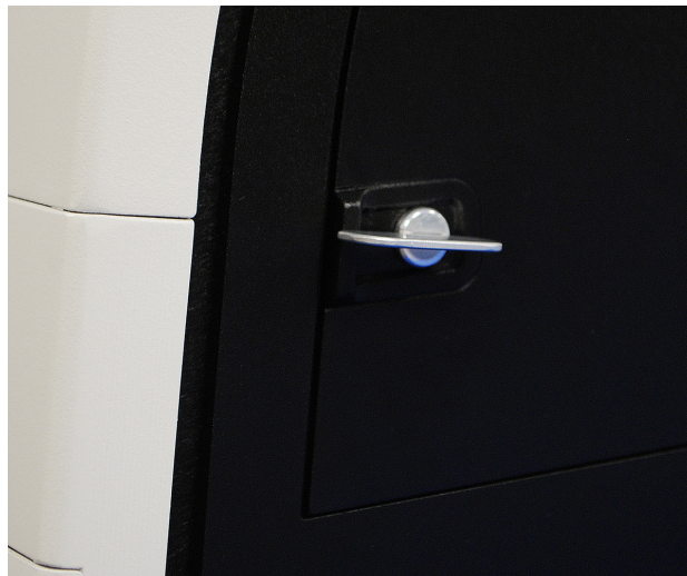
FIGURE 17. Door Access Tool Inserted and Turned
