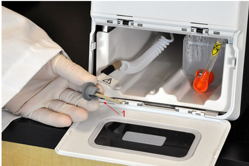
FIGURE 28. Pulling out the Drive Fluid Tube and Plug
